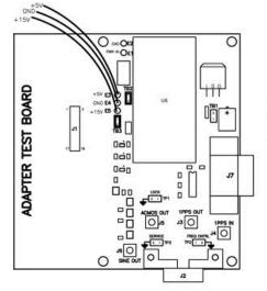
OPTION 2: +5V SUPPLIED TO E3 GND SUPPLIED TO E4 +15V SUPPLIED TO E5 TB2 AND TB3 ARE INSTALLED TB1 IS OPENED
