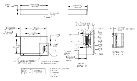
Note: The mating connector is a SAMTEC TMMH-109-01-G-DV-ES-A 2 X 9 shrouded header.
