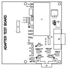
OPTION 3: J2 (26 PIN MOLEX) IS INSTALLED +10VDC TO +32VDC ARE SUPPLIED THROUGH PINS 1 THROUGH 7 TB1 IS INSTALLED TB2 AND TB3 ARE OPENED
