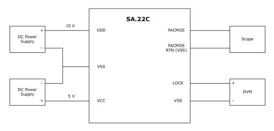
After the SA.22c starts receiving power, wait until the unit achieves atomic lock (typically 5 minutes). During this period, the monitored lock signal is HIGH. After the unit achieves atomic lock, the lock signal goes LOW.
